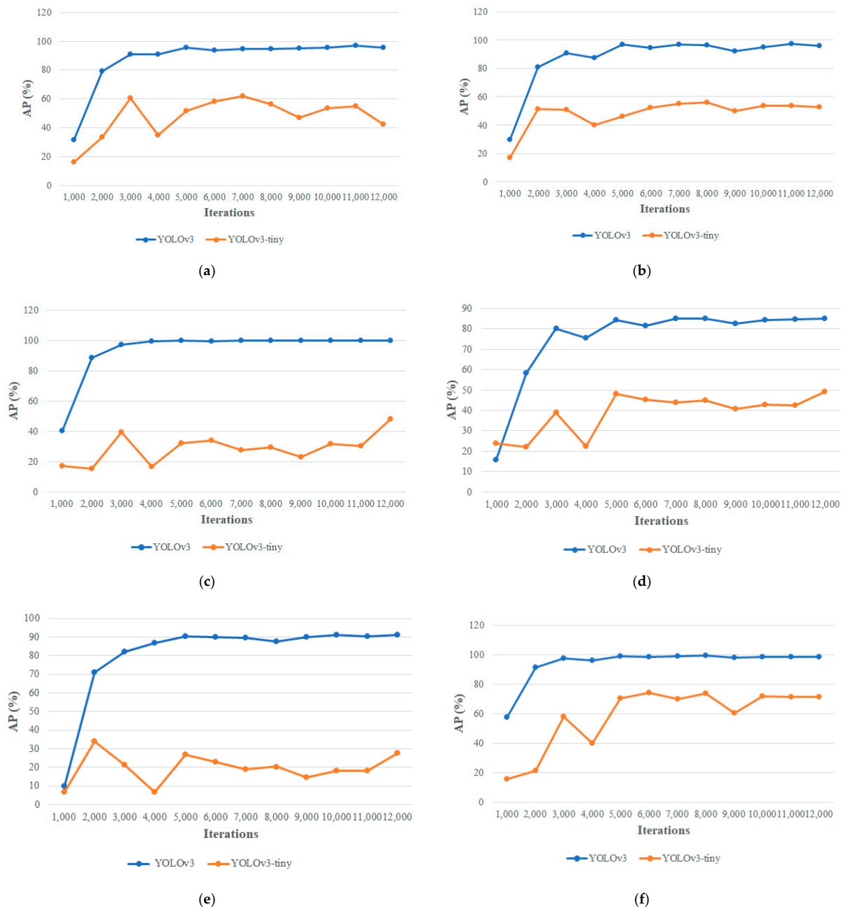
Figure 10. Variation in AP w.r.t. number of iterations for various classes via YOLOv3 and YOLOv3-tiny algorithm (a) cardboard (BD) (b) glass (NBD) (c) metal (NBD) (d) paper (BD) (e) plastic (NBD) (f) organic waste (BD).
