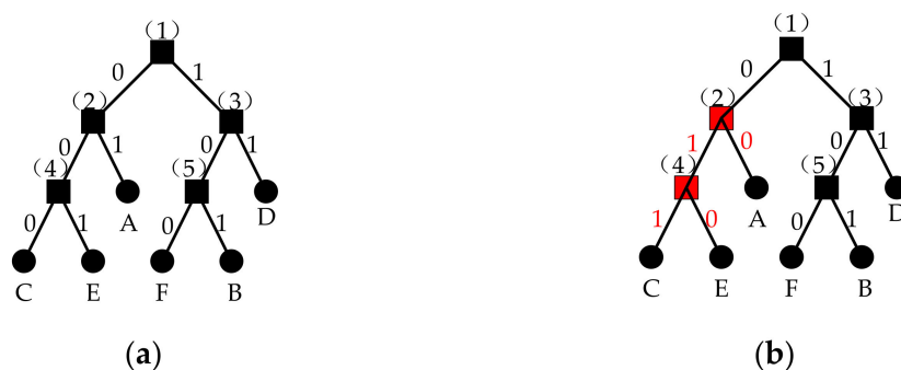
Figure 9. (a) Basic Huffman tree; (b) Mutated Huffman tree by changing the label-pairs of inner-nodes (2) (4).
