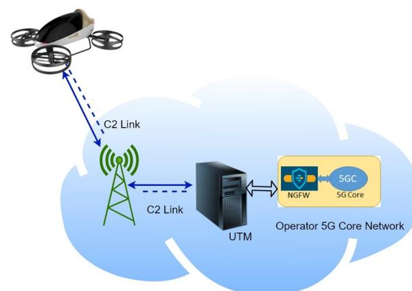
Figure 6. Cellular-connected autonomous UAVs controlled by UTM system.
