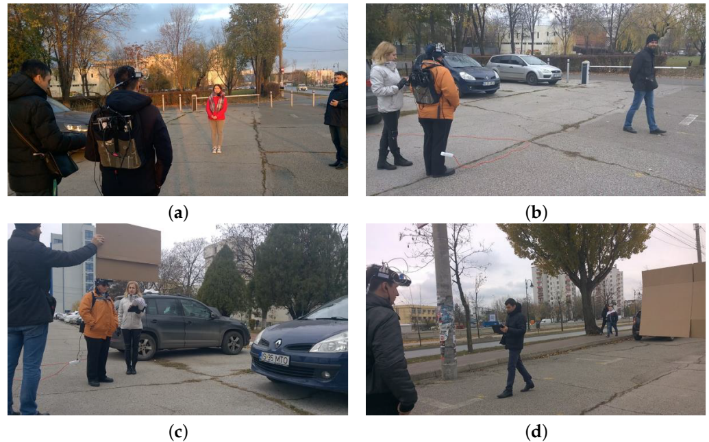
Figure 3. Examples of testing scene setups for perception tests with generic objects: (a) Scene with generic static objects (PT I-1); (b) scene with generic static and dynamic objects (PT I-2); (c) scene with generic static and elevated objects (PT I-3); (d) scene with generic static, dynamic and elevated objects (PT I-4).
