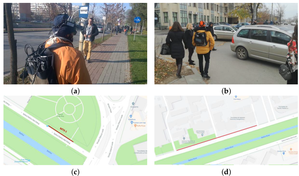
Figure 6. Examples of testing scene set ups for mobility tests in uncontrolled environments: (a) Walking on the sidewalk (45 m path), static and dynamic obstacles on the path, bus stop (MT II-1); (b) walking on the sidewalk (250 m path), static and dynamic obstacles on the path (MT II-2); (c) geolocation of MT II-1 testing scenario; (d) geolocation of MT II-2 testing scenario.
