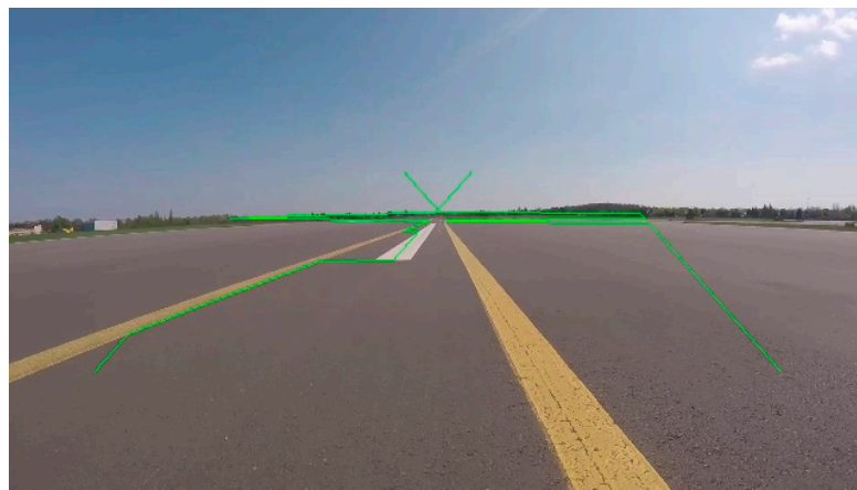
Figure 12. Result of running a program for line detection based on an edge detection algorithm.
