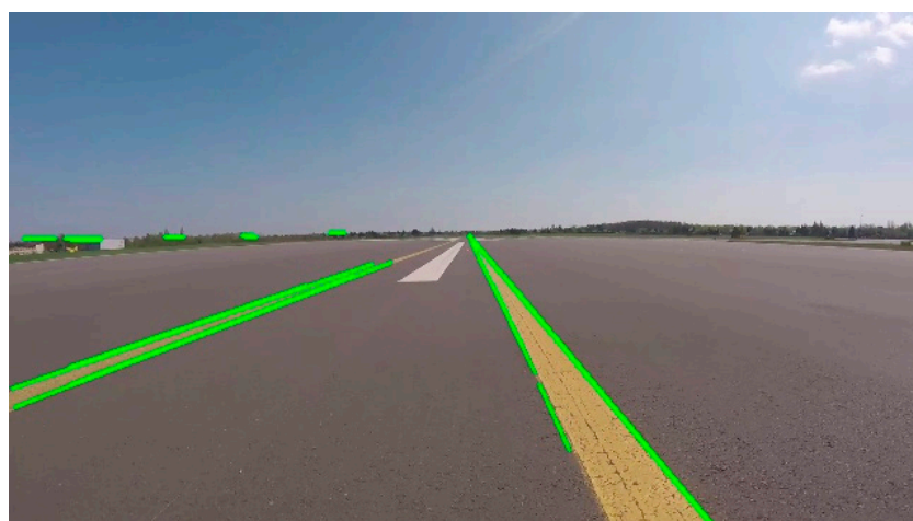
Figure 9. Result of program based on line detection using Scharr mask edge detection and Hough transform.
