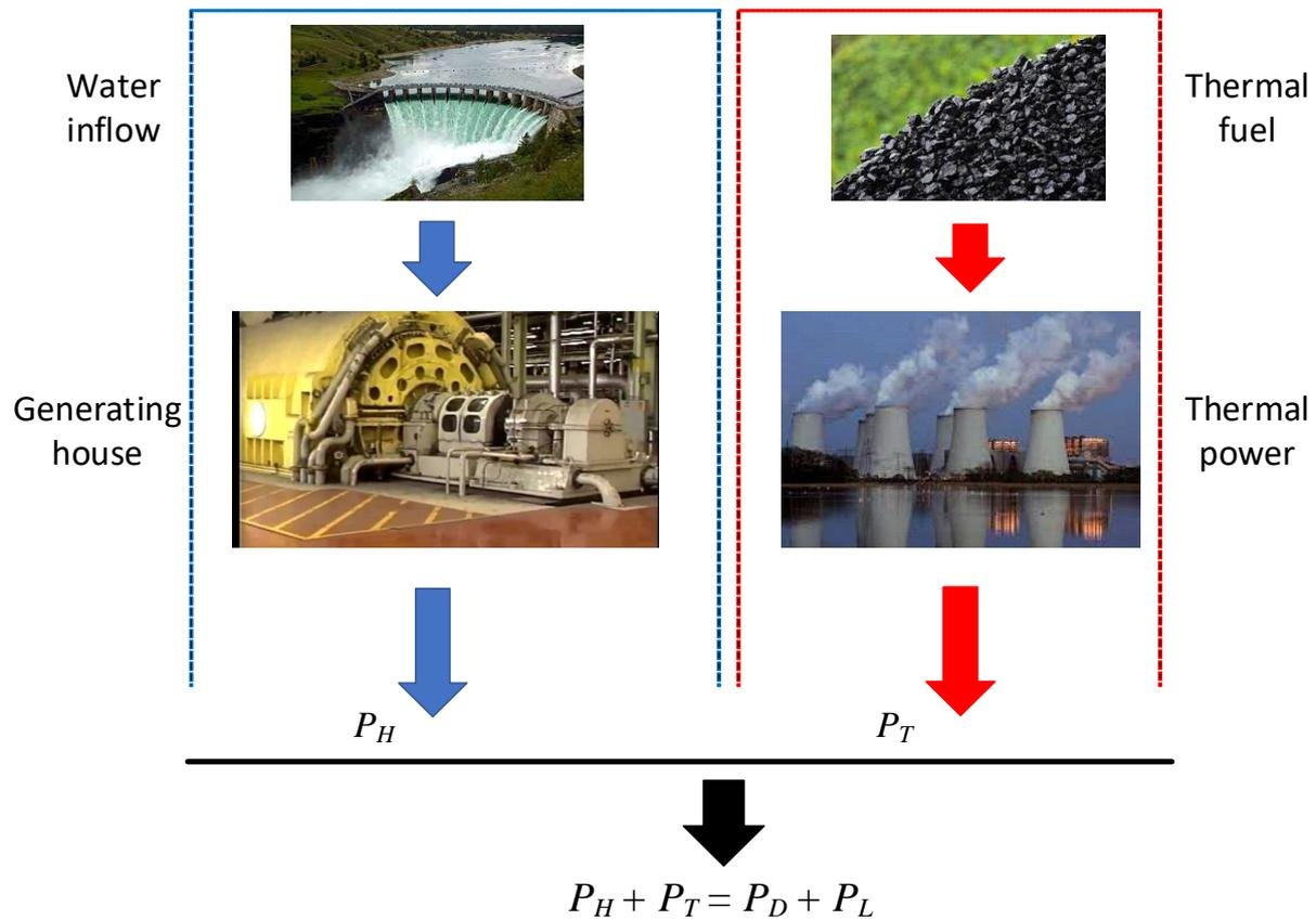
Figure 3. Block diagram representation for hydrothermal scheduling problem including single hydro and thermal unit.
