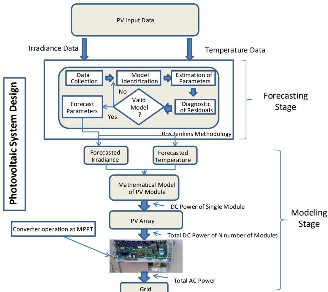
Figure 7. Basic flow chart for determining the PV power output for the economic dispatch problem.
