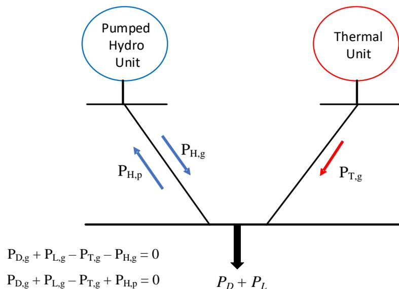
Figure 5. Equivalent circuit model of the pumped hydrothermal scheduling problem while considering the transmission losses of the system.
