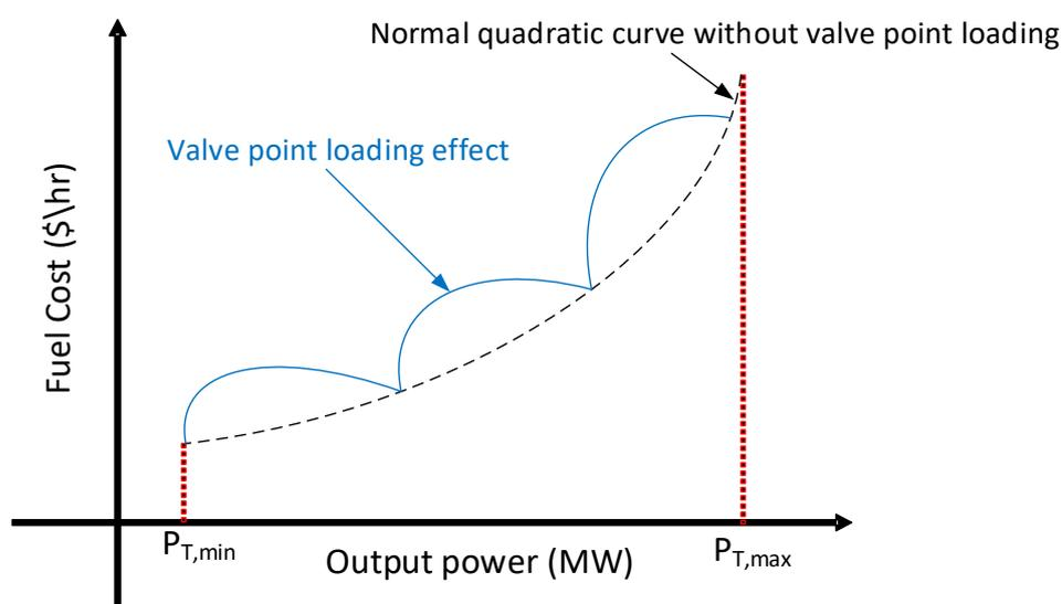
**Figure 2.** Comparison of the cost characteristics of thermal generators with and without valve point loading effect. The characteristics become non-smooth and contain bumps when the valve point loading is considered for thermal generators.
