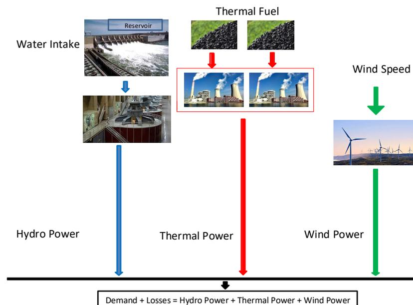
Figure 8. System configuration for the dispatch problem consisting of wind and conventional sources.
