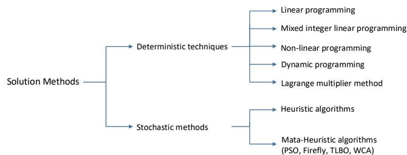
Figure 10. Breakdown of different solution methods used to solve various forms of the ED problem.
