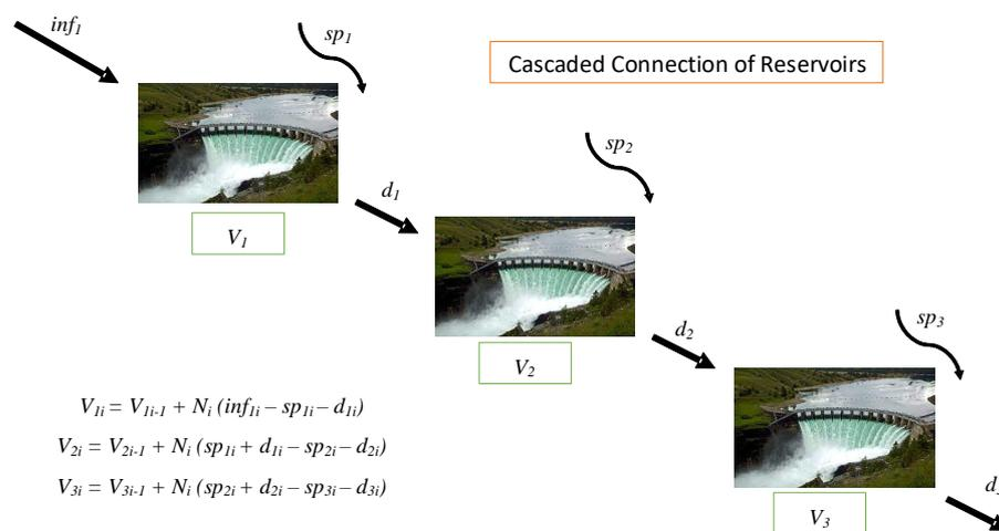
**Figure 4.** Block diagram representation for cascaded hydrothermal scheduling problem having reservoirs connected in a cascade connection.
