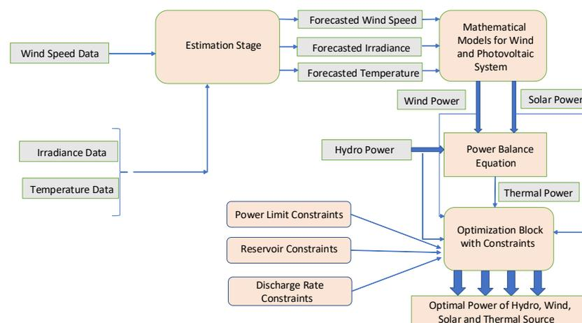
**Figure 9.** Overall block diagram for computing the dispatch problem for hybrid energy systems consisting of conventional and renewable sources.
