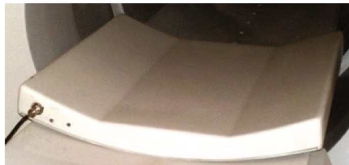
Figure 2. Sodium Whole Body coil. Reprinted by permission from Anisimov et al., App Magn Reson 2019 [23].
