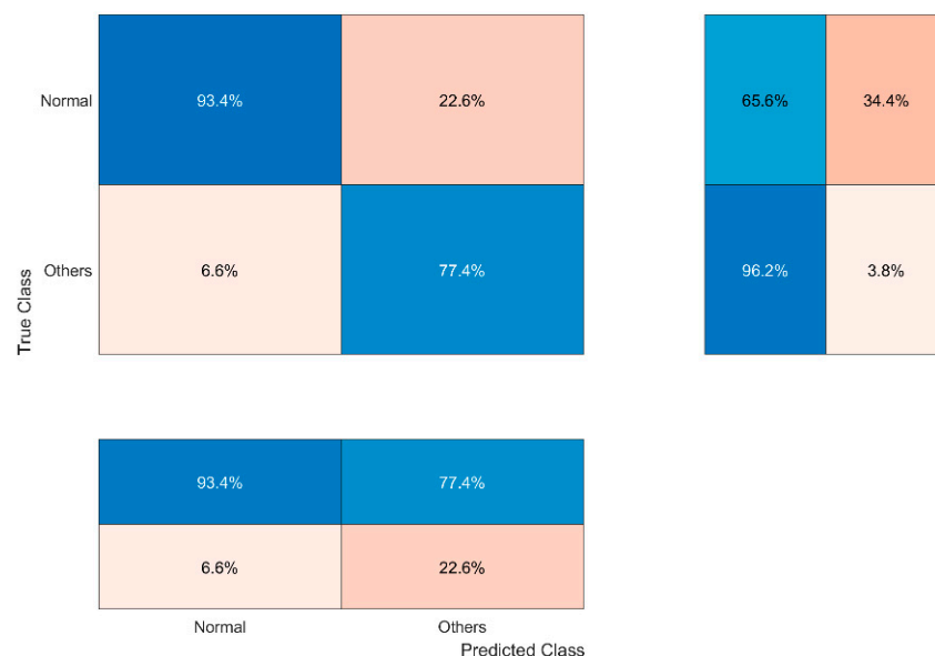
Figure 10. Confusion matrix of the first stage using ML.NET created model on UNSW-NB15 training dataset employing binary classification.
