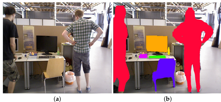
Figure 5. Segmentation effect: (a) the raw image; (b) semantic segmentation result.
