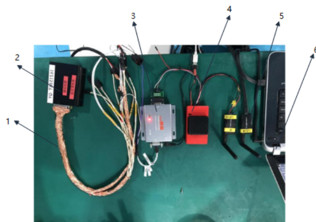
Figure 20. Joint debugging of flight control system and ECU. (1—ECU; 2—ECU harness; 3—RS-232 to TTL photoelectric isolation converter; 4—flight control board; 5—digital transmission platform; 6—ground station).
