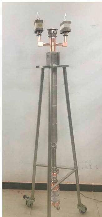
**Figure 13.** Prototype of the W-band  $TE_{02}$  mode gyro-TWT.
