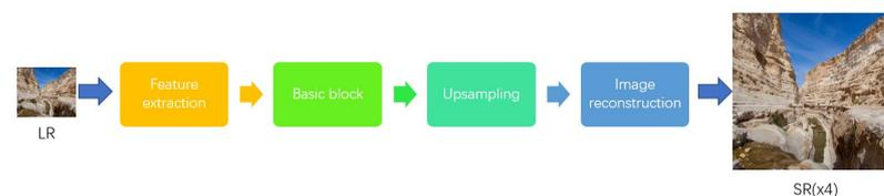
**Figure 6.** Super-resolution network framework (generator of GAN network).
