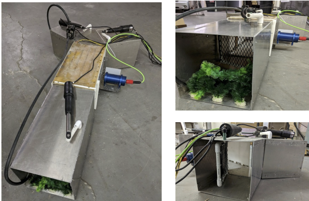
Figure 4. The design and dimensions of the four-chamber fish separation mechanism.
