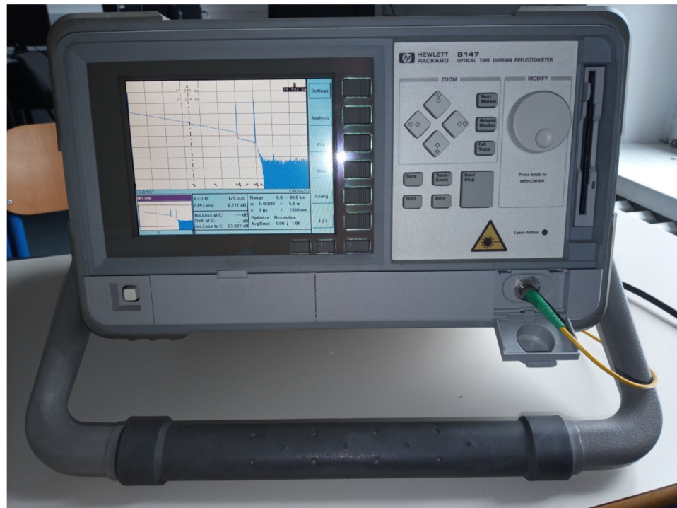
Figure 7. OTDR under test.
