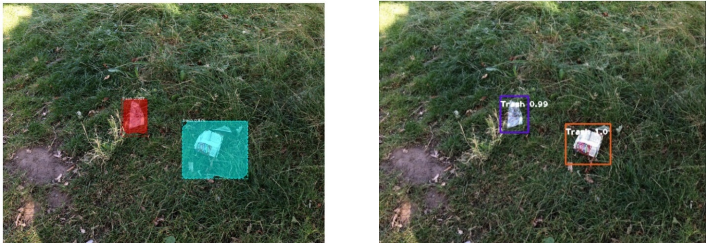
Figure 7. Trash detection using the custom Mask-RCNN model and trash detection using the custom YOLOv4 model.
