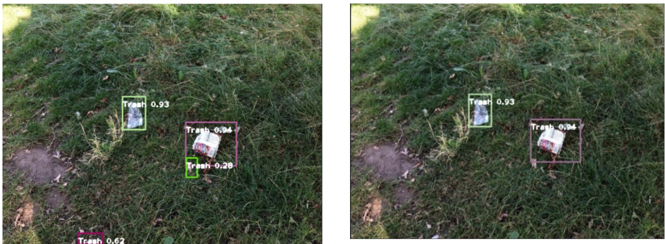
Figure 8. Trash detection using the custom YOLOv4-tiny model and trash detection using the YOLOv4-tiny model with minimum confidence for bounding boxes set to 0.7, i.e., 70%.
