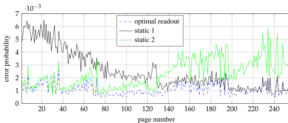
Figure 11. Error probability of a TLC block on r_7 (55 h bake, 3000 P/E) for optimal readout and 2 worst case static readouts.
