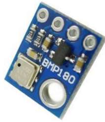
Figure 4. The BMP180 digital pressure sensor.
