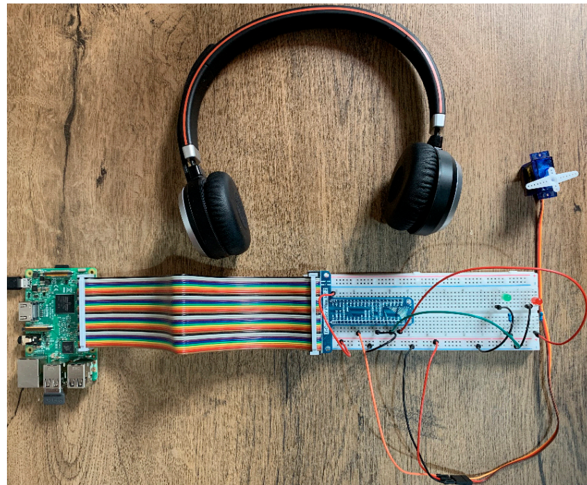
Figure 15. Real implementation of the voice control actuator using Bluetooth headphones for better comfort and freedom.
