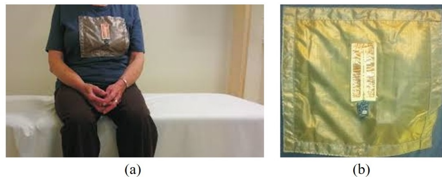
Figure 1. Wearable sensor settings during data acquisition: (a) positioning of the W^2ISP sensor on the subject's body, (b) the W^2ISP sensor attached to the subject's clothing with isolating silver fabric [47].
