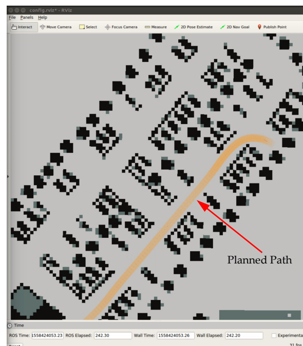
Figure 5. A visualization process of path planning on the parking lot created by RViz.
