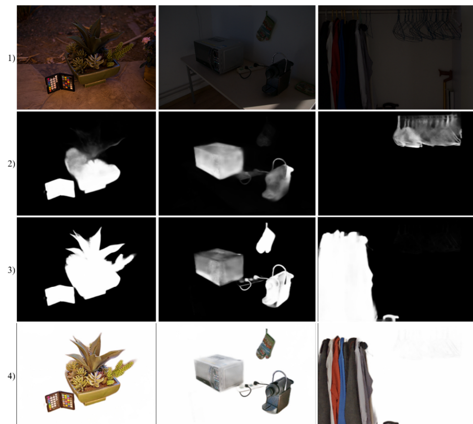
Figure 16. The results of salient object extraction model on the challenging LOL datasets. (1) low-light input images; (2) salient object extraction before image enhancement; (3) salient object extraction after image enhancement; (4) salient objects in full color space.
