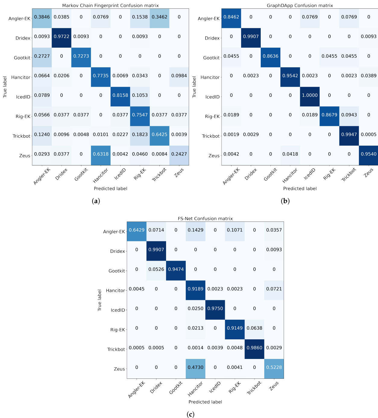
Figure 5. Confusion matrices of classification results using (a) Markov chain fingerprinting with maximum likelihood classifier, (b) traffic interaction graph with fully connected layer classifier (GraphDApp), and (c) embedding vector with FS-Net with balanced train set.
