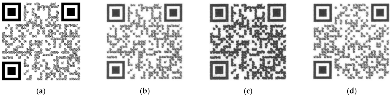
Figure 13. Example tags used to test the prototype system. (a) The original image of an authentic tag. (b) The scanned image of an authentic tag (printed version of image in (a)). (c) The scanned image of a counterfeit tag (cloned version of the authentic tag in (b)). (d) The scanned image of a forged tag.
