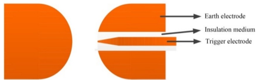
Figure 5. Schematic diagram of the trigger switch.
