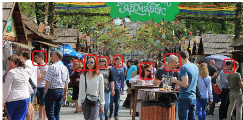
Figure 5. The face recognition algorithm applied to a frame of a crowd at a country fair. The average number of faces detected per frame is used to estimate the people density in the area. This public image has been chosen to illustrate the concept to be represented. In order to comply with data protection legislation, actual security camera footage has not been used.
