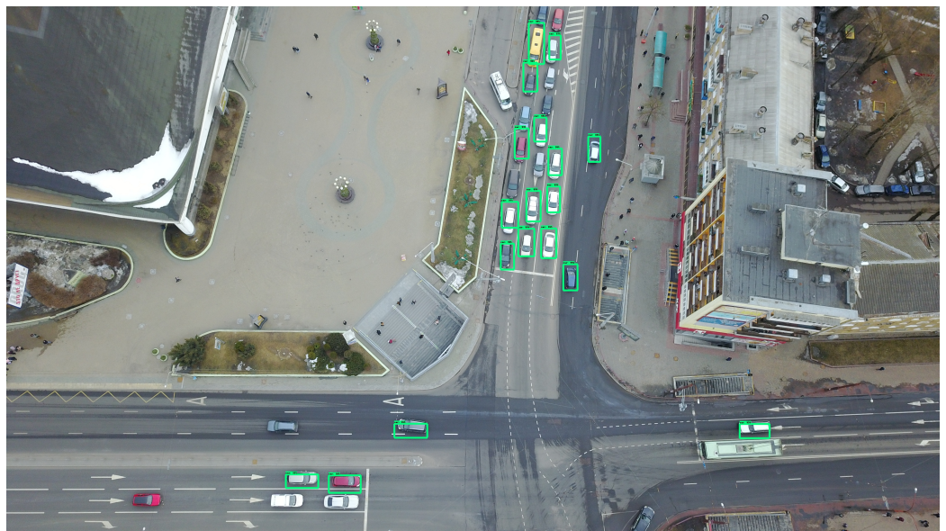
Figure 12. Example of Faster R-CNN misclassifications on an image of the PSU (Prince Sultan University) dataset, showing several false negatives (non-detected cars).
