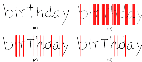
Figure 7. Segmentation based on vertical projection: (a) Original image, (b) image with segment lines after Step 1, (c) image with segment lines after Step 2, and (d) image with segment lines after Step 3.
