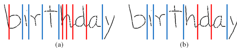
Figure 9. Over-segments removal: (a) Image with fixed and projection segment lines, and (b) image with correct segment lines.
