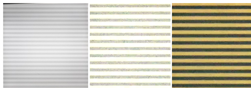
Figure 6. Rolling shutter effect: ROI of images containing an LED-based lamp switching at 1500 Hz, acquired with a rolling shutter camera at 25 fps with different frame resolution and environmental lighting conditions.
