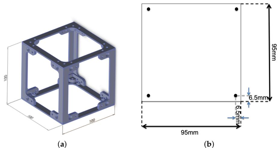
**Figure 3.** Structure and PCB measurements in mm. (a) CubeSat structure. (b) PCB size.
