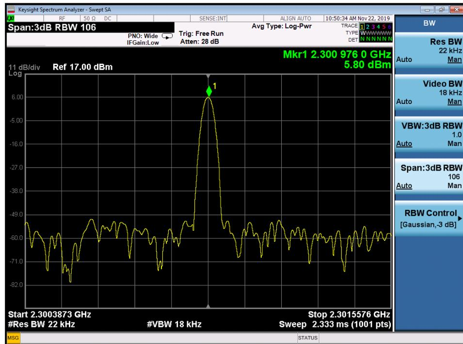
**Figure 12.** Spectrum radiated by RABE at 2.300 GHz. Image obtained from the signal analyzer with the prototype transmitting a single tone with a frequency of 2.300 GHz.
