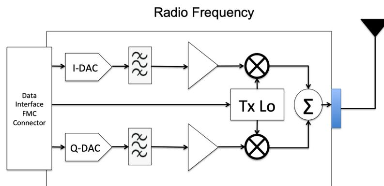
**Figure 2.** Radio frequency model. RF PCB scheme and AD9364 architecture.
