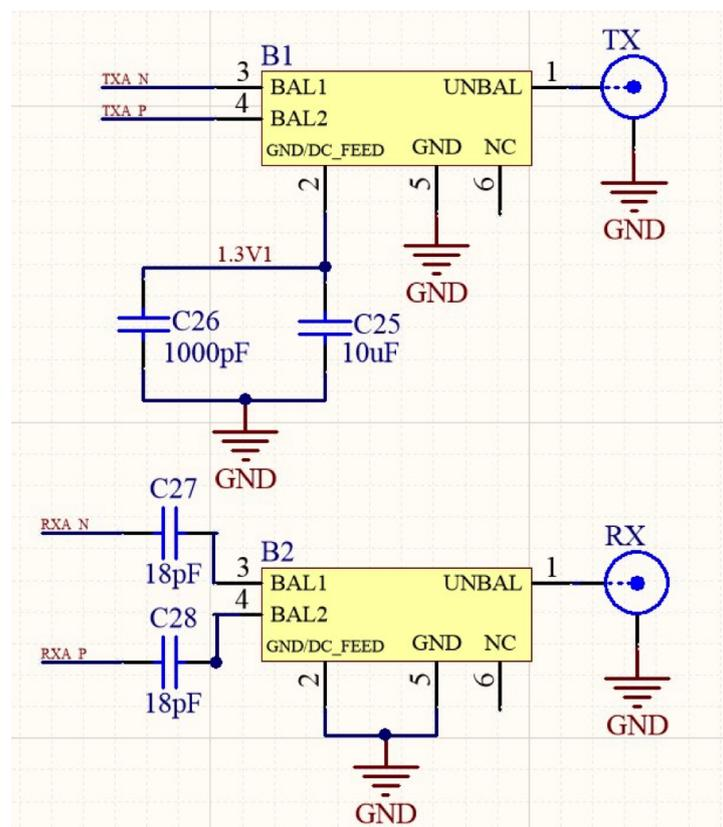
**Figure 6.** The RF matching stage, designed to avoid interference for 2–3 GHz.
