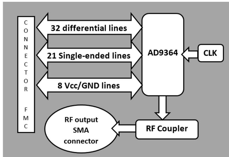
**Figure 4.** Schematic design of the RABE. This figure shows how AD9364 is connected to the FMC connector, as well as the FPGA and RF Output to the power amplifier stage (not shown at this work).
