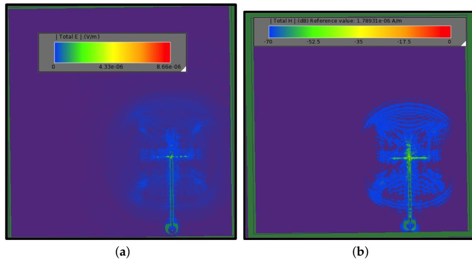
**Figure 13.**  $\vec{E}$  and  $\vec{H}$  field simulations on the RABE transmission line. (a) Electric ( $\vec{E}$ ) field. (b) Magnetic ( $\vec{H}$ ) field.
