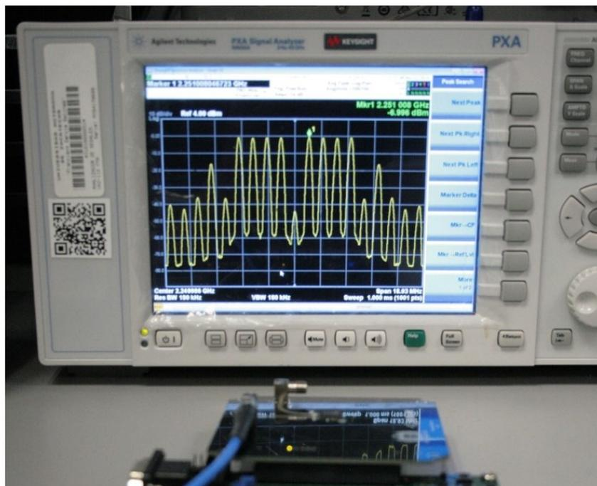
**Figure 11.** Signal analyzer, RABE and Zedboard on QPSK. The RABE prototype transmitting with 4-tone QPSK modulation, with 1 MHz frequency separations.
