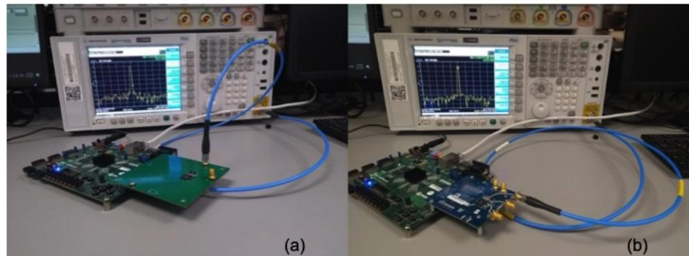
**Figure 9.** Implementation of the test bed for the RABE prototype. (a) tests of the manufactured prototype. (b) tests of the FMCOMMS4 card.
