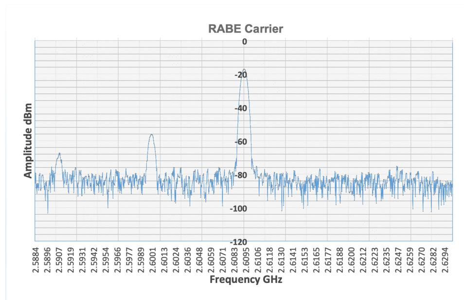
**Figure 10.** Spectrum of signal transmitted at 2.6095 GHz. Further processing of the data shows the spectrum of the carrier signal transmitted at 2.6095 GHz.
