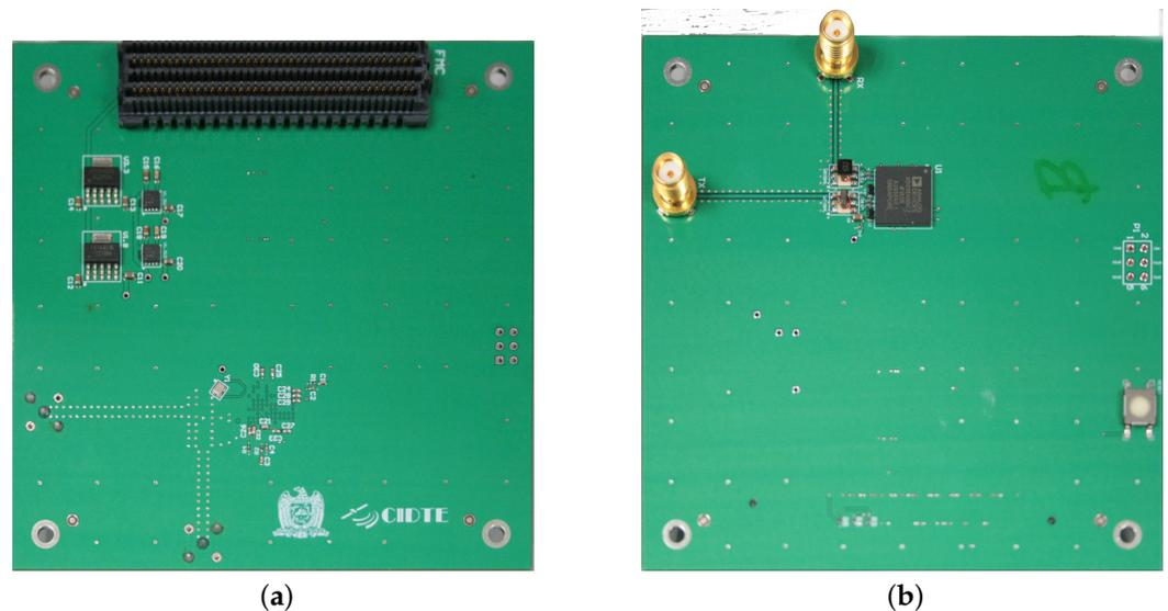
**Figure 7.** RABE-printed circuit board. A 3D model of the RABE ((a) top layer and (b) bottom layer).
