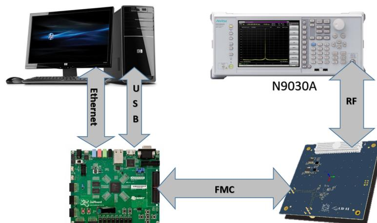
**Figure 8.** Testbed block diagram. Configuration for the connection of the test bed for the prototype.
