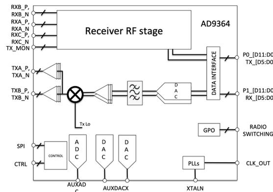
**Figure 5.** Block diagram of the IC AD9364. In this figure, the AD9364 manufacturer describes how it connects internally.
