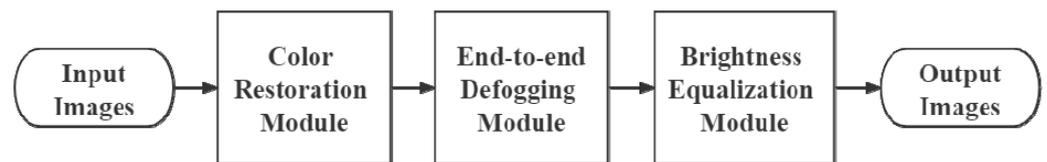
Figure 2. The process of the fusion algorithm.
