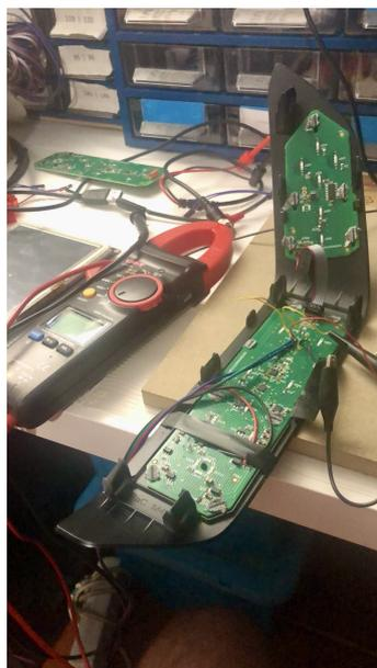
**Figure 5.** PCB with sensors based on a mutual-capacitance design assembled on a plastic part.
