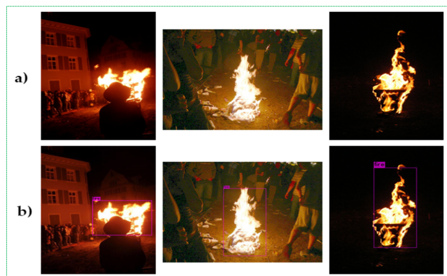
Figure 7. Visible experiment results in nighttime fire scenes: (a) input image sequences and (b) output image sequences with detected fire regions.
