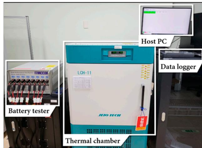
Figure 5. Battery experimental platform.
