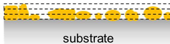
**Figure 6.** Conceptual picture of the GNP electrode layer and its division in three virtual layers of increasing Au volume from top to bottom.
