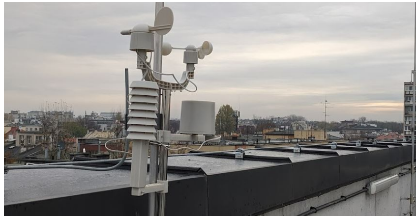
Figure 3. The SBS-WS-400 weather station mounted at the roof of the Institute of Telecommunications, selected as the reference one.
