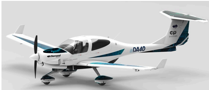
(a) eDA40 Diamond aircraft—All-Electric single engine trainer
