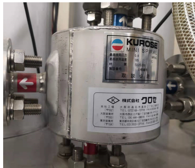
Figure A1. A spiral heat exchanger plant. Mini Spiral is a super compact spiral heat exchanger from Kurose Chemical Equipment Co., Ltd. in Japan. Design pressure is 0.6 MPaG. Design temperature is 185 °C. Material (JIS) is SUS316.
