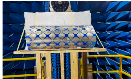
Figure 12. Test setup in the microwave anechoic chamber; the z-axis points to the top of the antenna.
