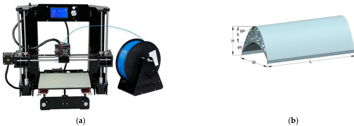
Figure 6. Three-dimensional printing device and dielectric material: (a) FDM printer; (b) printed substrate.
