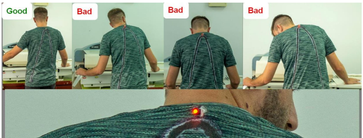
Figure 6. Assessed activity and wearable’s LED signaling when the person is in a risk-prone posture.
