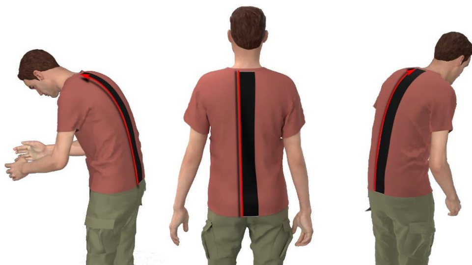
Figure 4. Placement and function of the motion sensor.
