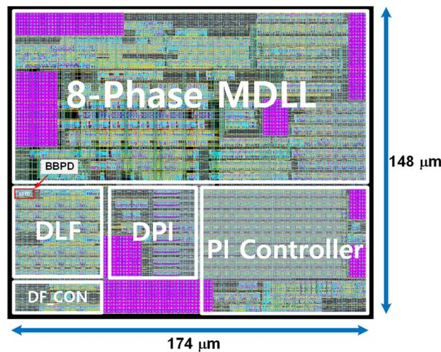
Figure 9. Chip layout of the proposed all-digital DJA.
