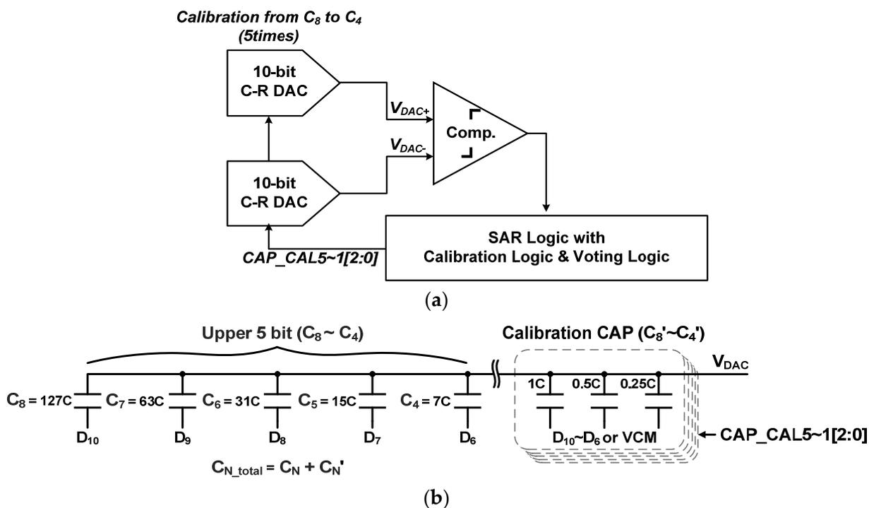
Figure 4. Calibration for upper 5-bit capacitors of C-R DAC: (a) concept; (b) block diagram.
