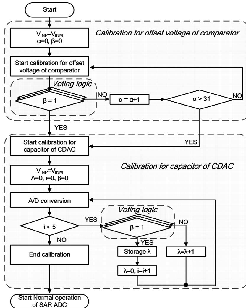
Figure 3. Sequence of C–R DAC calibration including comparator offset calibration.
