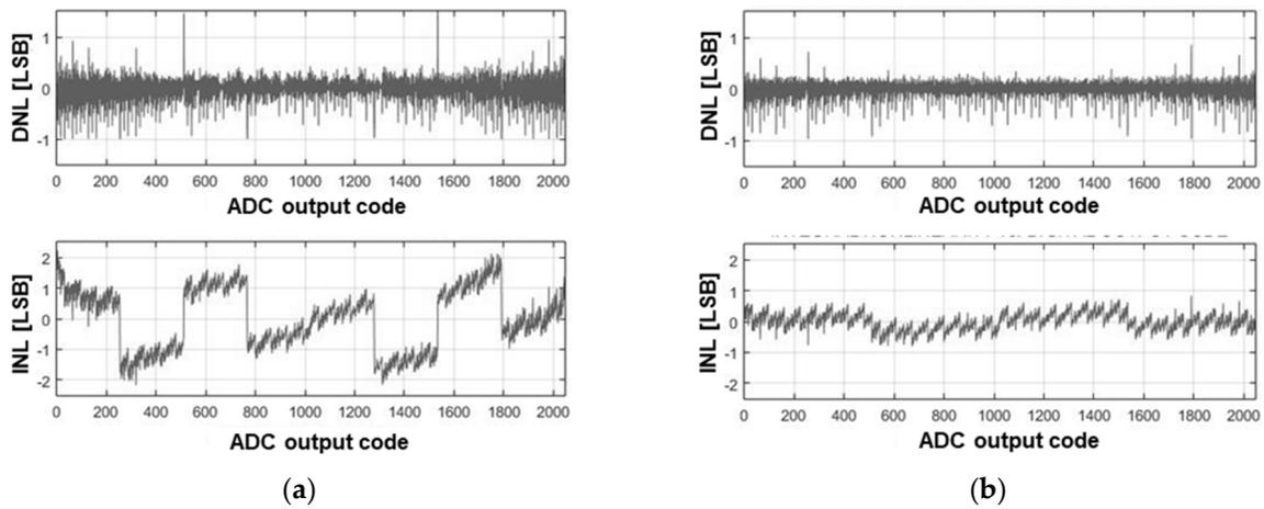
Figure 9. Measured static performances of 11-bit SAR ADC: (a) before C-R DAC calibration; (b) after C-R DAC calibration.
