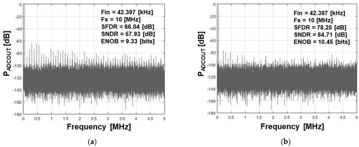
Figure 10. Measured dynamic performances of 11-bit SAR ADC at a differential analog input signal with low frequency of 42.39 kHz: (a) before C-R DAC calibration; (b) after C-R DAC calibration.
