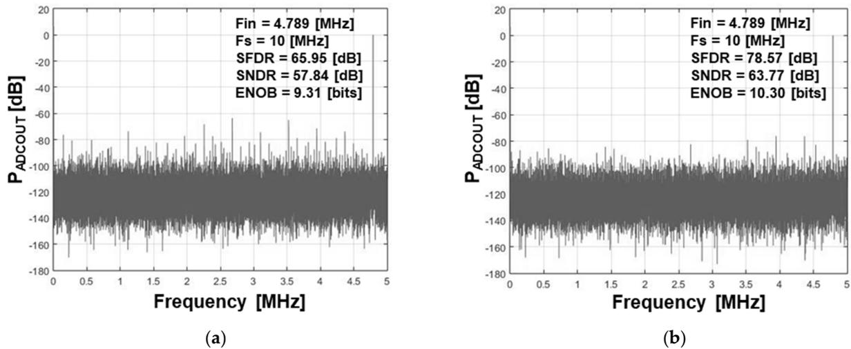
Figure 11. Measured dynamic performances of 11-bit SAR ADC at a differential analog input signal with Nyquist frequency of 4.78 MHz: (a) before C-R DAC calibration; (b) after C-R DAC calibration.
