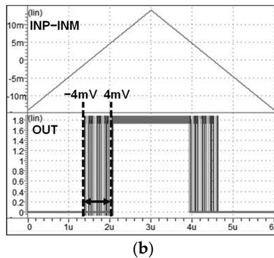
Figure 5. Comparator with offset voltage calibration: (a) circuit diagram; (b) simulation results.
