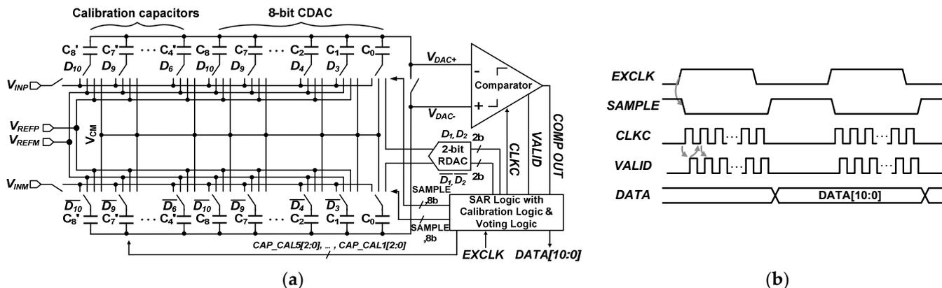
Figure 1. Proposed SAR ADC: (a) block diagram; (b) timing diagram.
