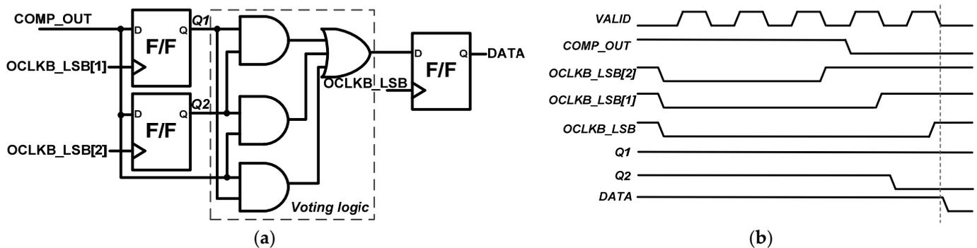
Figure 6. Voting logic: (a) block diagram; (b) timing diagram.
