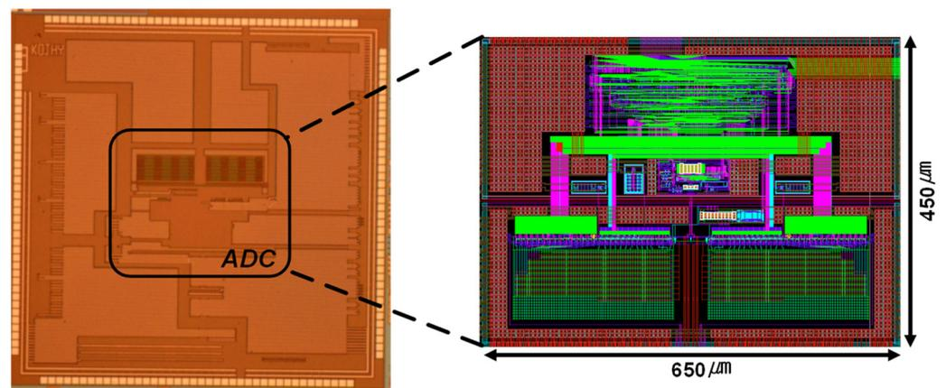
Figure 7. Chip photograph of implemented 11-bit SAR ADC.
