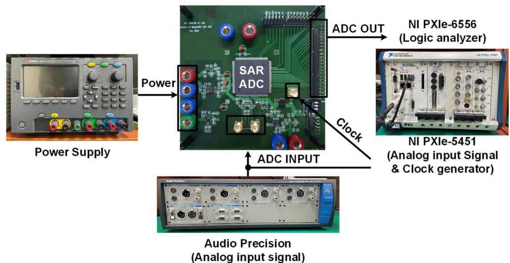
Figure 8. Test environment of implemented 11-bit SAR ADC.
