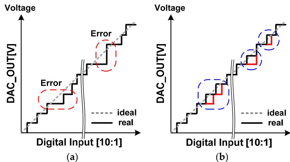
**Figure 2.** Transfer curves of CDAC: (a) with capacitor mismatch in CDAC; (b) after capacitor calibration in CDAC.
