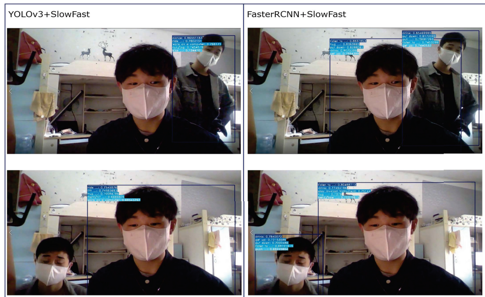
Figure 4. Comparison of YOLOv3+SlowFast and FasterRCNN+SlowFast in the same frame image detection effect.
