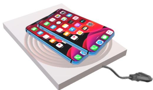
Figure 1. Wireless power transfer system with one transmitter charging multiple devices.
