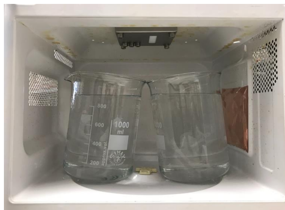
Figure 7. Picture of the antenna feeding the microwave applicator with the two water recipients set up for the IMPI test.
