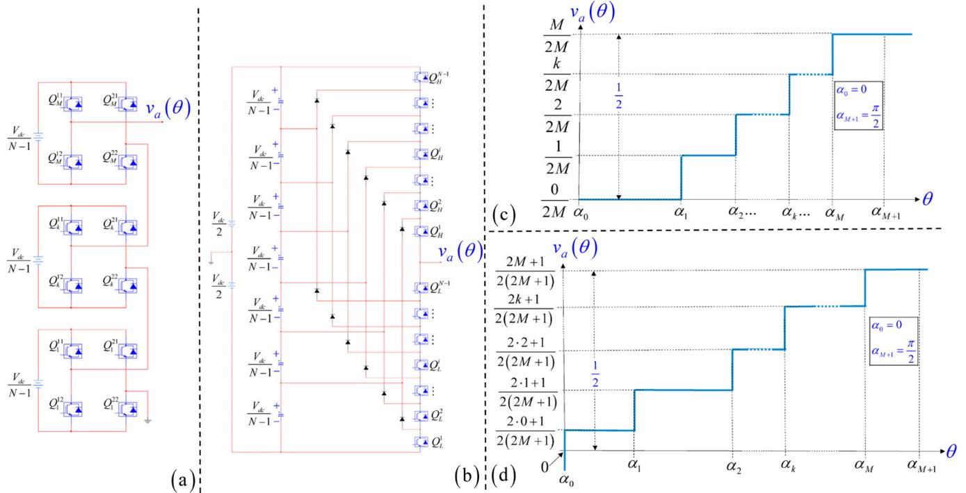
**Figure 1.** Generic MLI phase-leg: (a) cascaded H-bridge, (b) diode-clamped, and normalized odd quarter-wave symmetry SCM waveforms for: (c) odd-N case, and (d) for the even-N case.
