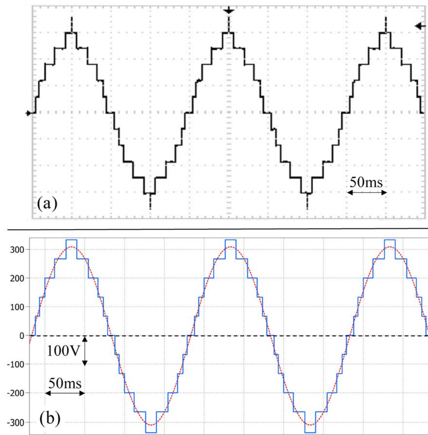
**Figure 11.** Line voltage SCM waveforms for  $m_a = 0.772$ . (a) Experimental results in [9], (b) corresponding processor-in-the-loop waveform with first harmonic indicated (dashed line).
