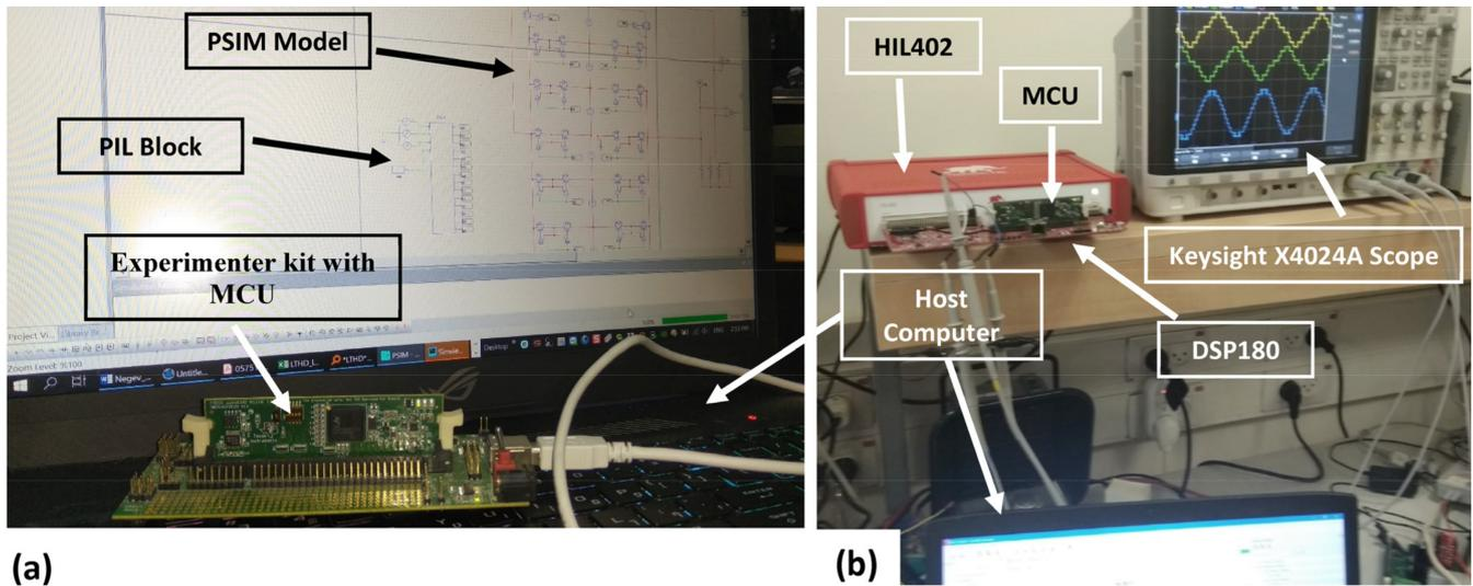
**Figure 10.** Real-time experimental setups: (a) processor in loop, (b) controller + hardware in loop.
