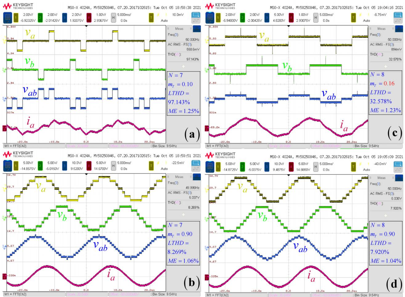
**Figure 12.** Real-Time experimental (C-HIL) results of optimal LTHD-based SCM (phase voltage, line voltage, and load current waveforms): (a) 7 Level CHB at  $m_T = 0.1$ , (b) 7 Level CHB at  $m_T = 0.9$ , (c) 8 Level DDC at  $m_T = 0.16$ , (d) 8 Level DDC at  $m_T = 0.9$ .
