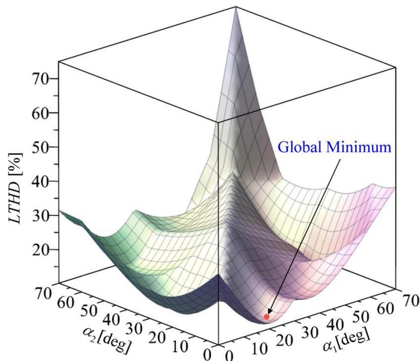
**Figure 4.** Analytical LTHD with global minimum for  $N = 5$ .
