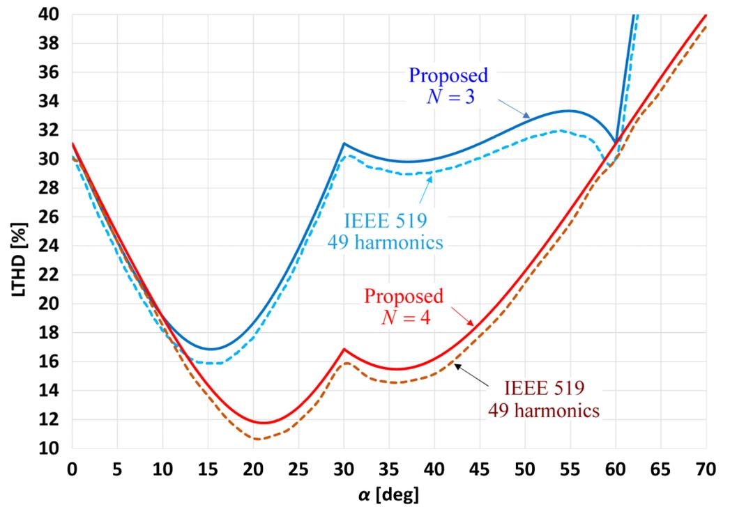
Figure 2. LTHD for  $N = 3, 4$ : proposed vs. 49 harmonics (IEEE 519 Std).
