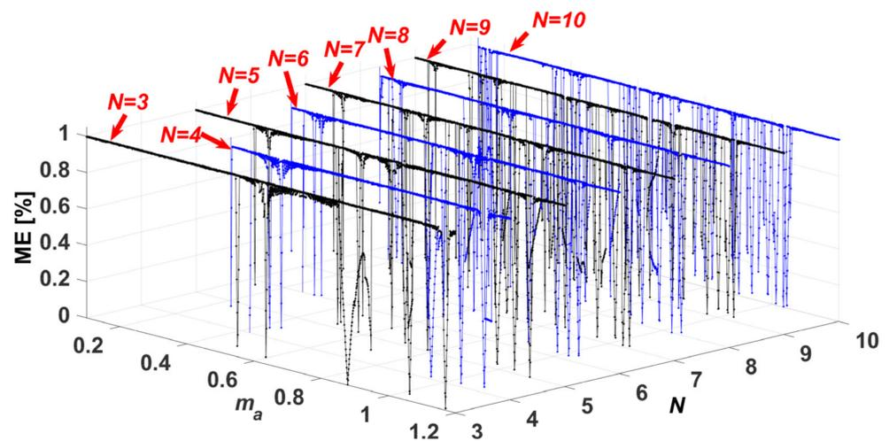
Figure 6. Calculated ME results for optimal LTHD vs. modulation index for various values of  $N$ .
