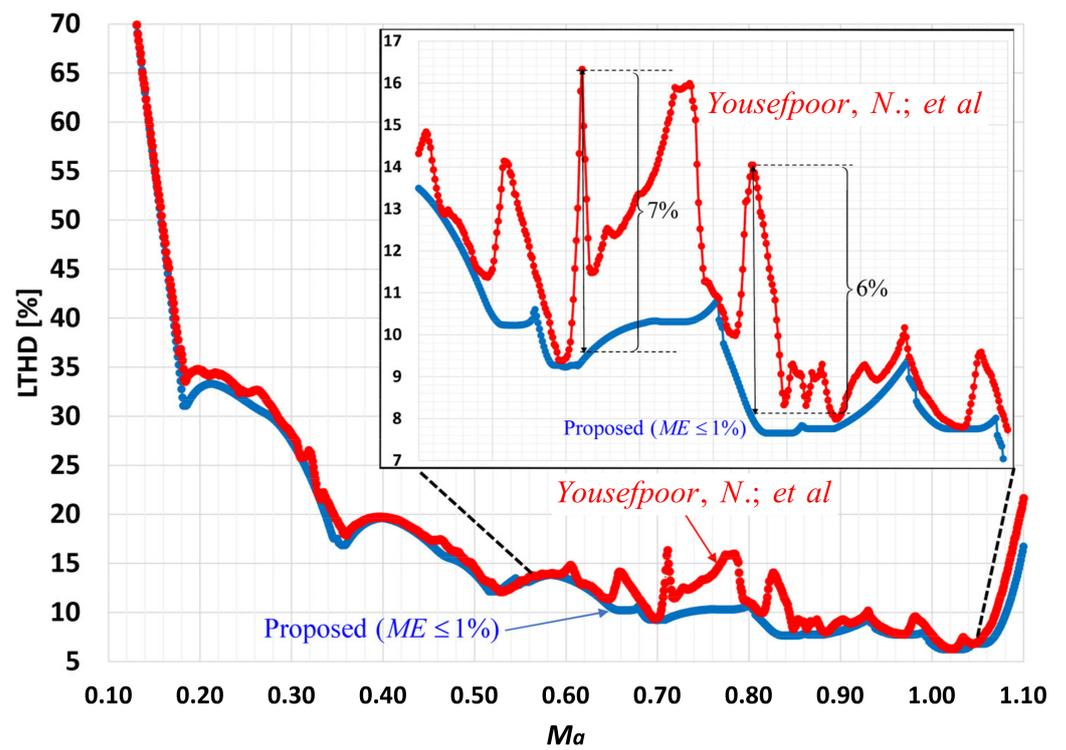
Figure 8. LTHD-optimal results (actual LTHD vs.  $ma$ ) for  $N = 7$ : analytical (proposed) vs. obtained in [9].
