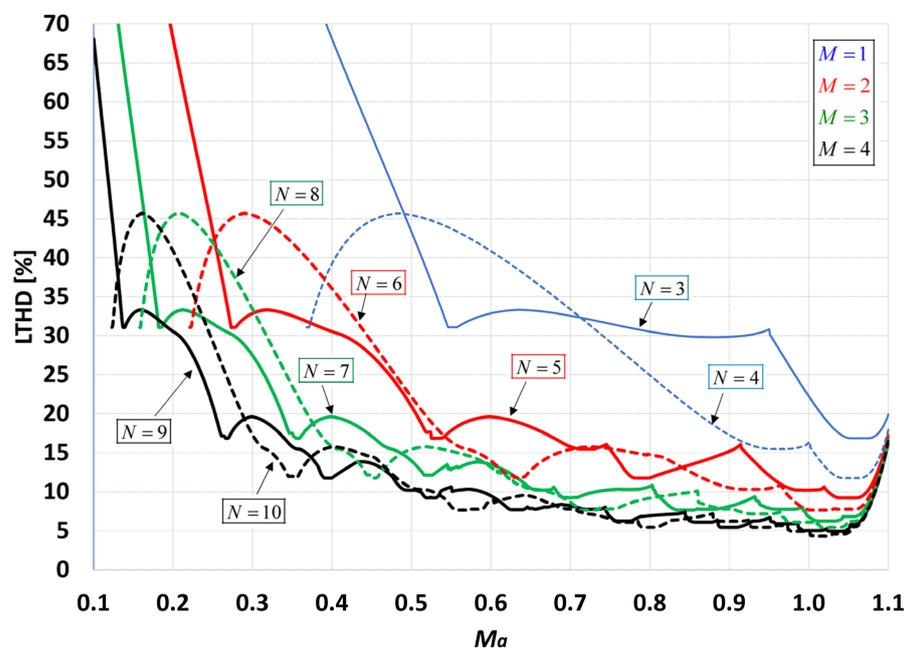
Figure 5. Calculated minimum LTHD vs. modulation index for various values of  $N$ .
