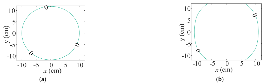
Figure 10. Zero coupling position of M_{23} at a clearance of (a) \Delta Z = 10 cm and (b) \Delta Z = 16 cm.
