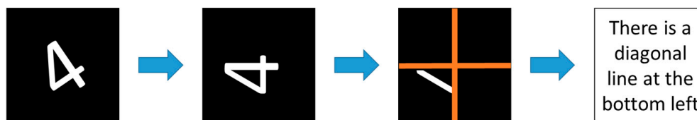
Figure 11. Tilt correction example of "4".
