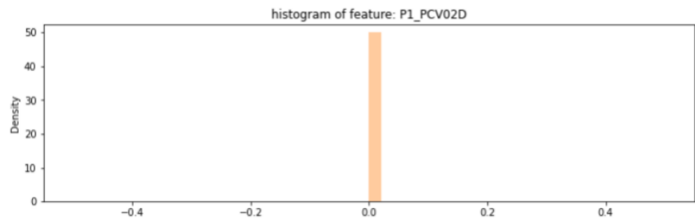
Figure 8. Feature graph for data point P1_PCV02D. This feature graph means that the values of the data points do not change over time.
