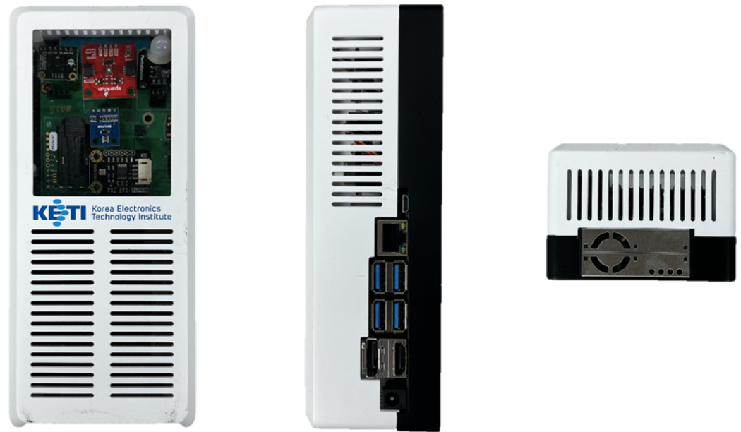
Figure 1. Intelligent multi-environment sensor module: (left) front of the module (center), side of the module, and (right) top of the module.
