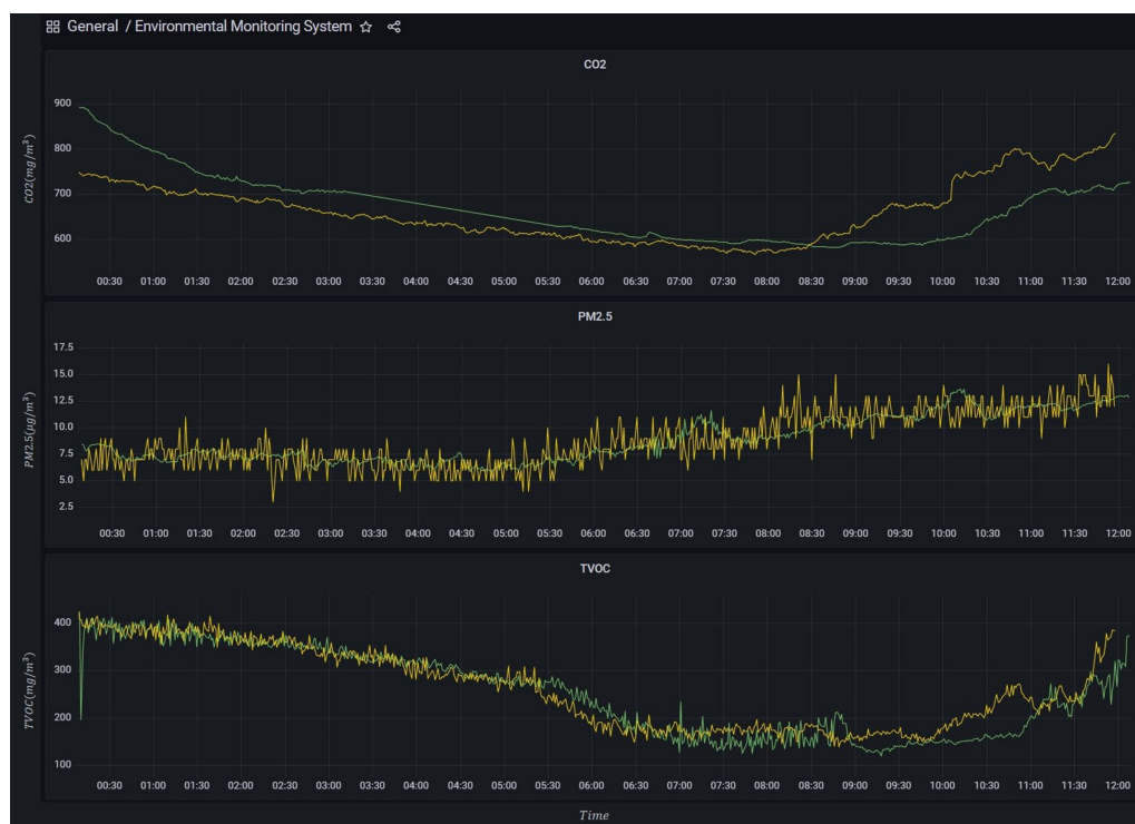
Figure 10. Indoor air quality monitoring system (CO 2 , PM 2.5 , and TVOC). Green line: predicted data; yellow line: actual data.
