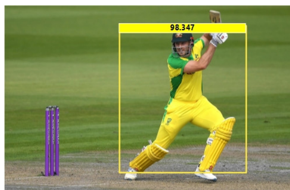
Figure 5. Bounding box showing detected person after application of aggregated channel features algorithm.
